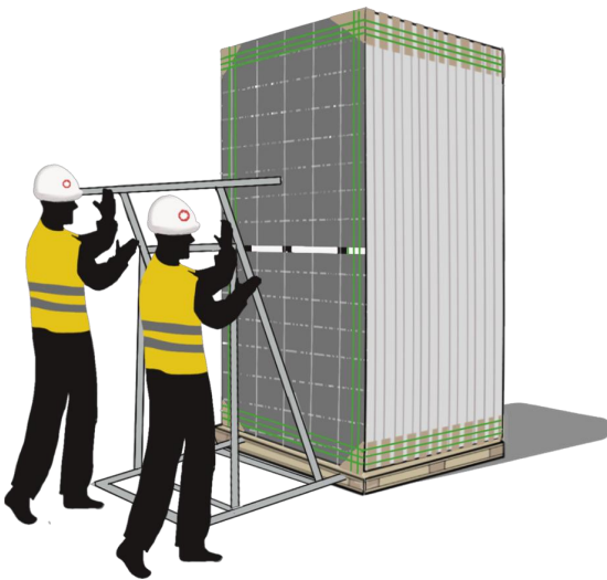
③ Place the stand supporter from the glass or backsheet side.
