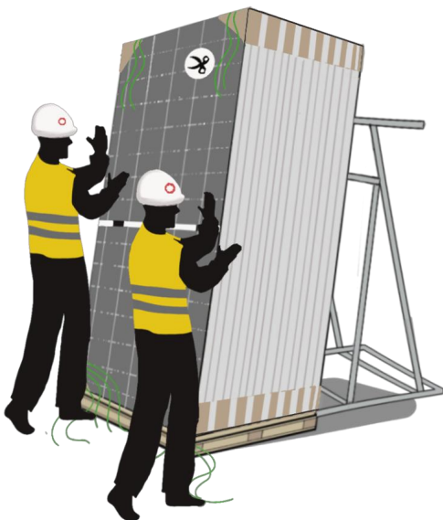
⑤ Cut off the remaining packing belts so that the modules rest on the stand supporter.
