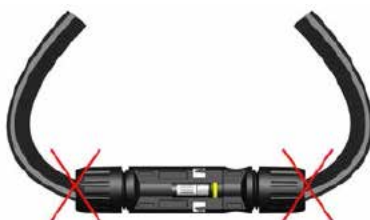
Wrong bending method
